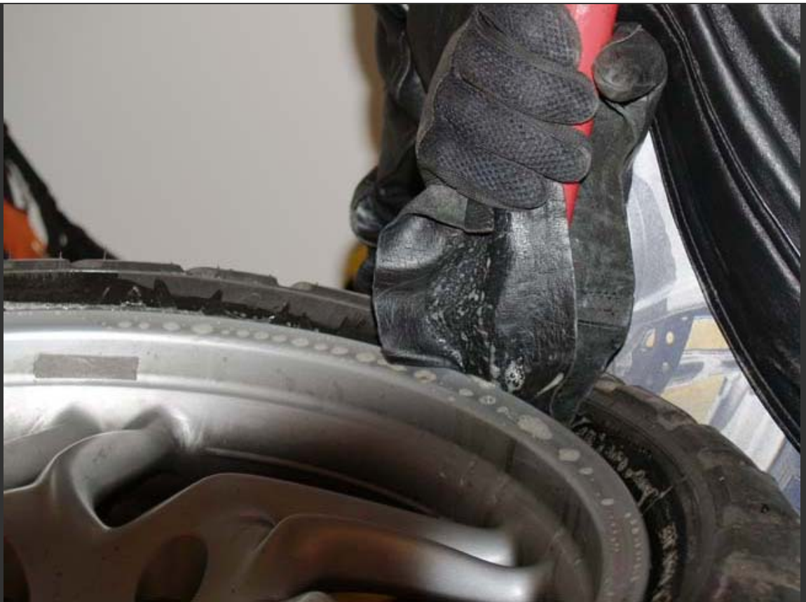
Insert the thin end of the bar in between the tire and rim.
