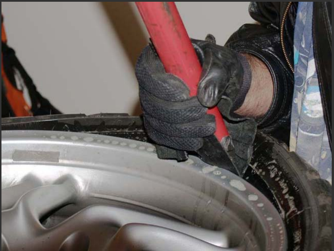
Catch the lip of the bead on the tire and pull the bar over.
